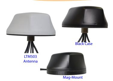
Mobile Mark's LTM503 Series Multiband Diversity/MIMO antenna contains five separate antennas, all in one compact antenna housing: two broadband LTE/Cellular antennas, one dual-band WiFi antenna, one Iridium® antenna and one GPS antenna. The LTM503 differs from the LTM501 in that it covers the Iridium frequencies from 1616-1626.5 MHz.
