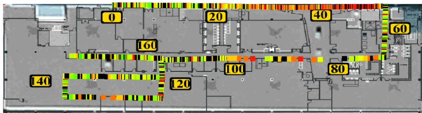
Figure 4: Throughput Heat-map, MIMO via 2-port CMX antenna.
