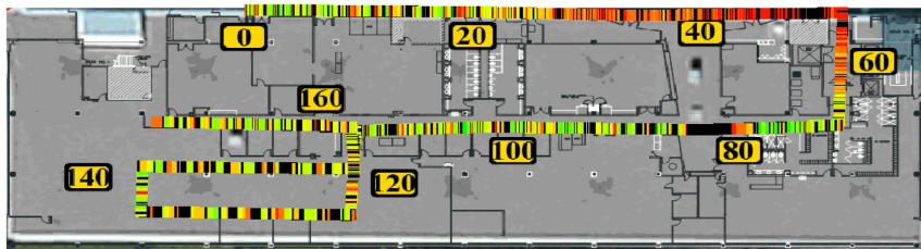
Figure 3: Throughput Heat-map, MIMO via 2-port MIMO CMD antenna.
