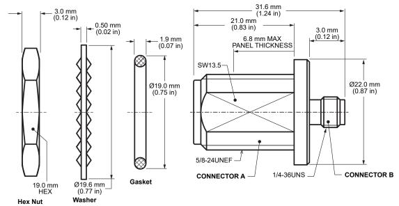
Figure 1. Product Dimensions for the ADP-SMAF-NF-B-W Adapter
