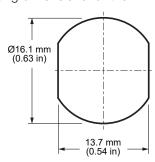
Figure 2. Recommended Enclosure Mounting Dimensions
