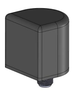
he RFMAX RKD-44 series antenna is designed to replace a single cellular antenna with a DUAL 4G/LTE antenna in the same 5/8 inch mounting hole. This unit is purpose built to be ultra-rugged and tamper proof which makes it ideal for use in public places. A VHB gasket seals the mounting location from water ingress, and 5/8 threaded mounting stud provides a completely vandal proof design.
