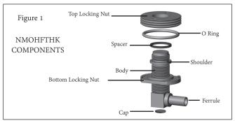
NOTE: The NMOHFTHK comes with a spacer which allows the mount to be used with a variety of antenna designs. Remove the spacer when using the mount for all products with the SuperSeal Gasket. When not using the SuperSeal Gasket (using just the O-ring) or for products not supplied with a SuperSeal Gasket, use the spacer
