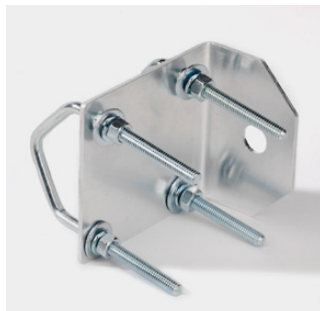
BAM1009 Antenna Mount Aluminium L-bracket for horizontal or vertical mounting on pipes or masts. Suitable for pipes and masts with 38 - 60 mm outer diameter. Hole with 15.8 mm diameter for mounting with N(f) connectors.
