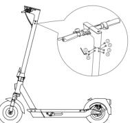
2. Install the handlebar on the front tube in the correct direction.
