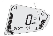
Gear position display (first gear shown)
