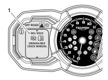
If when attempting to activate the hill hold control system, the message HILL HOLD UNAVAILABLE - CHECK MANUAL is displayed, this indicates one or more of the following:
