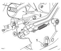
l. Oil drain plug 2. Oil filter
