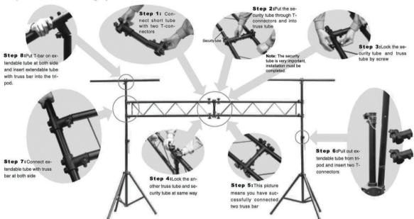
This trussing system offers easy set-up and high stability. It comes complete with two tripods that telescope to nine feet featuring two locking grooved pins. Also included are two T-bars and two five foot truss that securely lock together to create 10 feet of trussing span, or they can be used seperately. This trussing system is excellent for mobile DJs, bands, and rentals. Never overtighten any of the connectors.
