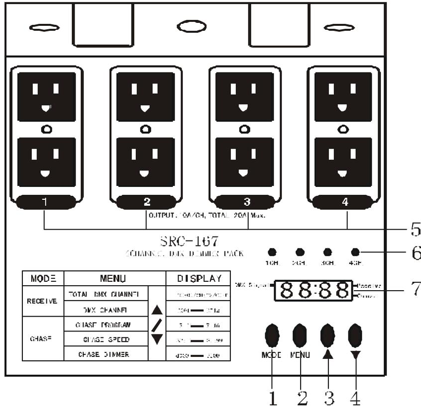
1. Mode button - this button will change the power packs operate mode between DMX and chaser.
