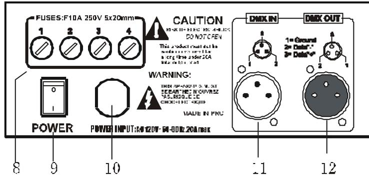
8. Channel fuses - each of the four channels is protected by 10A (120V) or 6.3A(230V) fuse. These fuses prevent you from overloading and damaging your pack. Be sure to always replace with the exact same type fuse.
