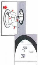
Release the mounting springs and the retrofit luminaire will now be partially installed in the recessed can housing.
