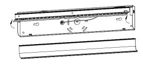
Position the housing in the desired location then mark and drill mounting holes at the narrow ends of the keyhole slots. Screw in mounting screws leaving space for housing thickness. Slide housing over mounting screws, shift into position and tighten screws.
