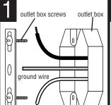
ATTACH cross bar to outlet box with outlet box screws (8-32 x 1/2, 2 slotted screws provided).
