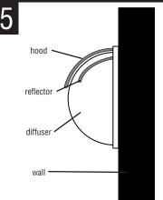
ON MODELS WITH HOOD, attach to wall with reflector up. Hood is to be placed above reflector as shown.
