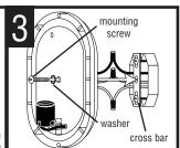
POSITION THE FIXTURE over the outlet box and secure in place with the mounting screw (1/4-20 x 1,1 provided). Screw lamp into lampholder. Use lamp type and wattage specified on fixture
