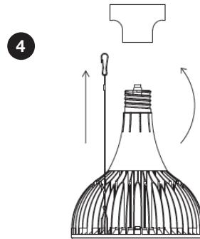
NOTE: The lamps must be operated in a base up position. Not for horizontal operation.
