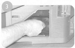
Remove the lamp door. Turn the knob counterclockwise to the OPEN position and pull out the door.
