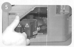
Insert the new lamp unit, paying attention to the orientation and direction of insertion. Ensure that the new unit is mounted securely. If the lamp is not reattached securely, the self-diagnostic function may be triggered and the POWER/STANDBY indicator will flash three times.
