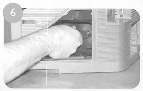
Reinstall the lamp door. Secure the door by turning the knob clockwise back to the CLOSE position.
