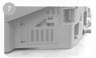
Replace the outside lamp cover. Plug the power cord back into the wall outlet and turn on the power.
