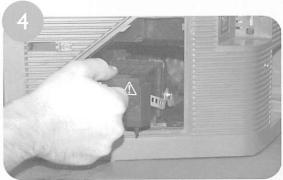
Remove the lamp unit from the television by hooking a finger through the loop of the lamp handle and pulling it upwards; pull the lamp straight
