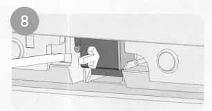
Insert the new lamp unit, paying attention to the orientation and direction of insertion. Ensure that the new unit is firmly seated. **Note:** To avoid shortened lamp life and/or reduced picture quality, do not touch the glass portion of the new lamp.
