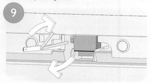
Tighten the screw firmly on the new lamp unit, taking care not to overtighten.
