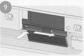
Replace the lamp cover by pushing it back on. **Note:** Ensure that the cover is mounted correctly and securely, otherwise the self-diagnostic function may be triggered and the POWER/STANDBY indicator will flash three times.
