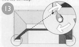
Tighten the screw on the rear side panel. Plug the power cord back into the wall outlet and turn on the power.
