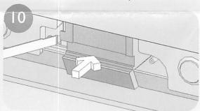
Replace the lamp cover by pushing it back on. **Note:** Ensure that the cover is mounted correctly and securely, otherwise the self-diagnostic function may be triggered and the POWER/STANDBY indicator will flash three times.
