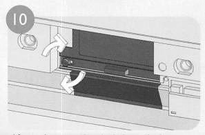
After making sure that the hole on the lamp cover aligns with the hole on the lamp unit, reattach the lamp cover by tightening the screw.
