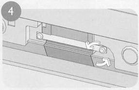
Loosen and remove the right screw on the lamp cover.
