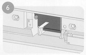
Remove the lamp unit from the television by pulling it out. Dispose of lamp in accordance with disposal laws. **Note:** To avoid injury, exercise caution when removing the lamp unit and do not place your hand in the lamp storage area.
