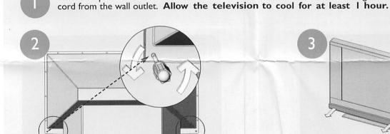
Loosen the screws on the rear side panel.
