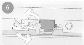
Loosen the screw securing the lamp.
