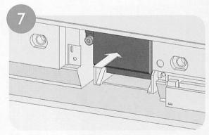
Insert the new lamp unit, paying attention to the orientation and direction of insertion. Ensure that the new unit is firmly seated. **Note:** To avoid shortened lamp life and/or reduced picture quality, do not touch the glass portion of the new lamp.
