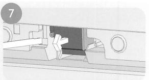
Remove the lamp unit from the television by pulling it out. Dispose of lamp in accordance with disposal laws. **Note:** To avoid injury, exercise caution when removing the lamp unit and do not place your hand in the lamp storage area.
