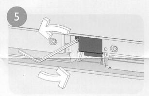
Loosen the screw securing the lamp.
