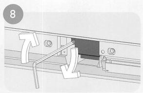
Tighten the screw firmly on the new lamp unit, taking care not to overtighten.
