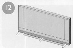
Replace the front panel by aligning it on the television.
