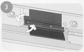
Loosen and remove the left screw on the lamp cover.
