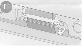
After making sure that the hole on the lamp cover aligns with the hole on the lamp unit, reattach the lamp cover by tightening the screw. **Note:** For proper lamp operation, ensure that the screw is inserted correctly.
