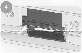
Slide the knob to the left and remove the lamp cover.
