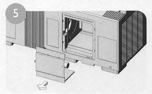
Remove the lamp unit from the television by grasping the handles and pulling straight out. Slowly remove the entire lamp assembly unit from the television. Dispose of lamp in accordance with disposal laws.
