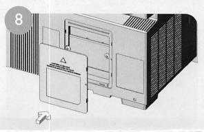
Replace the lamp access door. First, insert the catch tabs into the slots on the left side of the lamp access compartment. Press the door until it is fully closed and the latches are engaged. Tighten the screw using a screwdriver.
