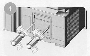
Using a screwdriver, loosen (but do not remove) the two screws on the lamp unit.
