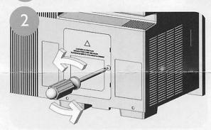
Locate the lamp unit access door and review the listed precautions. Loosen (but do not remove) the screw located on the door.
