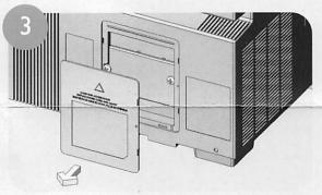
Press the catch tabs to remove the entire lamp access door. One catch tab is located above the loosened screw, the other is below. Remove the door and place to the side.
