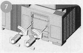
Tighten the two screws firmly on the new lamp unit, taking care not to overtighten.
