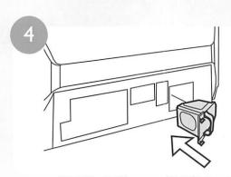
Insert the new lamp unit, paying attention to the orientation and direction of insertion. Ensure that the new unit is firmly seated. Tighten the two screws securing the lamp cartridge, taking care not to overtighten.
