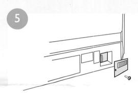
Replace the outside lamp cover; replace the screw securing the cover.
