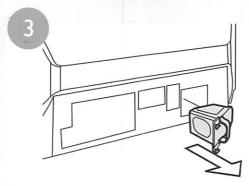
Loosen (but do not remove) the two screws securing the lamp unit. Remove the lamp unit by grasping the handle and pulling straight out. Dispose of the lamp in accordance with disposal laws.
