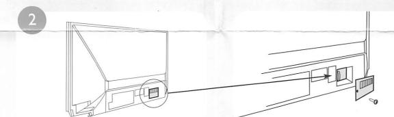
Using a Phillips head screwdriver, loosen and remove the screw securing the outside lamp cover; remove the cover.
