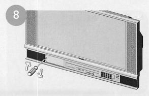
Replace the lamp cover by re-engaging the two clips; tighten the screw on the lamp cover.
