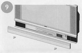
Replace the front cover by aligning it on the television and pushing gently until it snaps into place. Plug the power cord back into the wall outlet and turn on the power.
