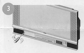
Using a Phillips head screwdriver, remove the screw securing the lamp cover; remove the cover.
