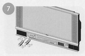
Tighten the screws firmly on the new lamp unit, taking care not to overtighten.
