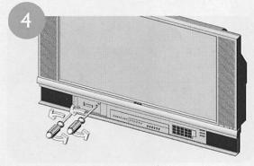
Remove the two screws on the lamp unit.
