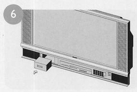
Insert the new lamp unit, paying attention to the orientation and direction of insertion. Ensure that the new unit is firmly seated.
