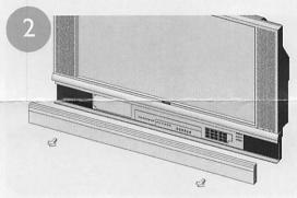
Remove the front cover of the television by pulling it outwards until the snap unlatches.
