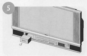
Remove the lamp unit from the television by grasping the handle and pulling straight out. Slowly remove the entire lamp assembly unit from the television. Dispose of lamp in accordance with disposal laws.
