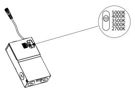
6 Connect driver wire to fixture wire, ensuring the connectors are properly aligned and fully screwed down.
