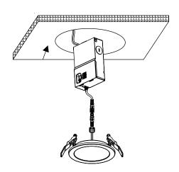
8 Lift both retention tabs upwards, insert into hole, and press fixture upward until it sits flush against the ceiling.
