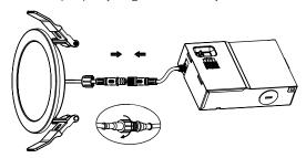
If using extension cables, insert cable between driver and fixture ensuring the connectors are properly aligned and fully screwed down.
