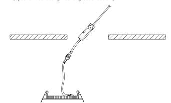
Push up spring-arms on side of fixture, lift into ceiling, and release spring-arms.
