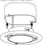
Turn fixture to lock into keyholes. Tighten two (2) screws.
