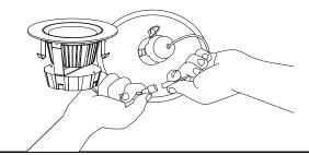
4 Align friction clips with recessed housing.
