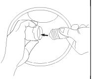
3 Plug the downlight connector into the Edison (or GU24) base connector.
