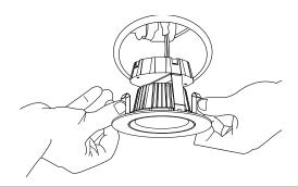
5 Carefully route wires into housing and push the downlight upward, flush to ceiling surface.
