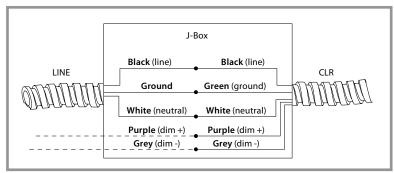
**NOTE:** If 0-10V dimming is NOT to be connected, it is recommended to cut off the exposed, tinned leads on the purple and grey wires, and cover the ends with a small piece of electrical tape or wire nut. If bare 0-10V control wires should accidentally touch a grounded surface, it could cause unintended flickering or dimming of the light fixture.
