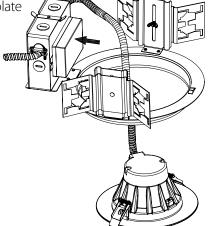
6 Lift upward on retention tabs while pushing the retrofit kit through the rough-in, release the retention tabs and push trim flush to the ceiling, ensuring a secure fit.
