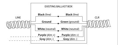
**NOTE:** If 0-10V dimming is NOT to be connected, it is recommended to cut off the exposed, tinned leads on the purple and grey wires, and cover the ends with a small piece of electrical tape or wire nut. If bare 0-10V control wires should accidentally touch a grounded surface, it could cause unintended flickering or dimming of the light fixture.
