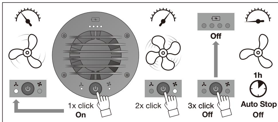
AirZing UV-Compact operates continuously when plugged in through USB TYPE-C cable and a 5V / 3A charger.
