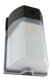
Sunlite 88169-SU LED Outdoor Mini Wall Pack Light Fixture, 25 Watts (200W Equivalent), 120-277 Volts, 3000 Lumens, Built-In Photocell, 50,000 Hour Life Span, ETL & DLC Listed, 3000K Warm White
