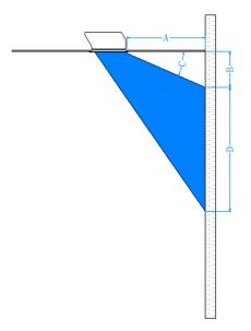
Step 2. Ceiling opening: The product needs a 585mm\*585mm ceiling opening. Drill the opening at the installation positions calculated in step 1.
