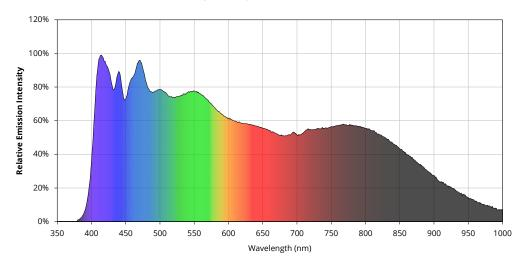
This LED was developed to provide broad wavelength coverage, flat spectral shape and high radiant flux density for scientific research and industrial inspection applications.
