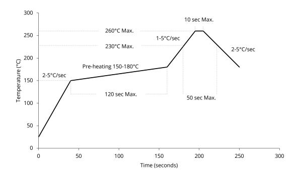
Note: Soldering paste with the melting point at 230  $^{\circ}\text{C}$  is recommended.
