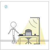
▶ When motion is detected with approach of a human, this lamp auto-activates and perform lighting condition of its previous time.
