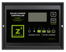
For use with 12/24Volt Solar Panel; Suitable for Solar panels up to 760 Watts on 12V mode: 1520Watt on 24V mode
