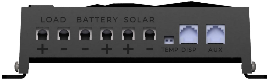
Figure 4: Bottom of CINDER 40 Showing All Connections
