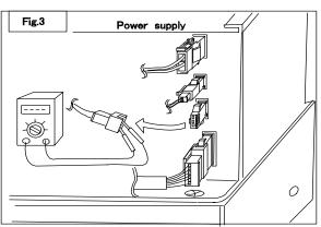
Note ) Compressor runs continuously when you make to short circuit at this coupler.
