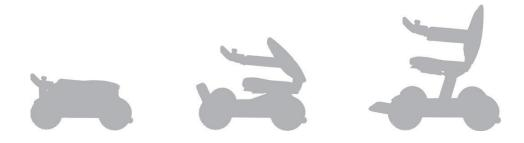
Expanding scooter, if there is no other command, it will stop automatically after unfolding
