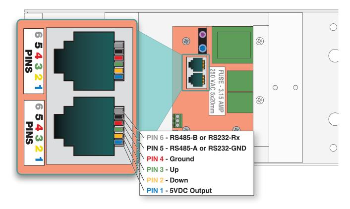
Section 6 - Wiring LVC-IV to Motor
