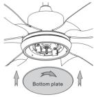
If light is not required, remove globes and replace glass shade diffuser with metal cover.
