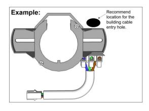
NOTE: Ensure building cable will enter the canopy close to terminal block. DO NOT enter the building cable direct on top of the hanging ball area.
