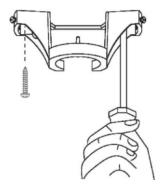
**NOTE:** Ensure building cable will enter the canopy close to terminal block.
