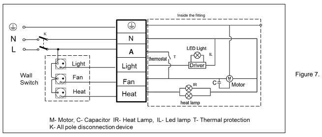
The wiring diagram is shown on Figure 7.
