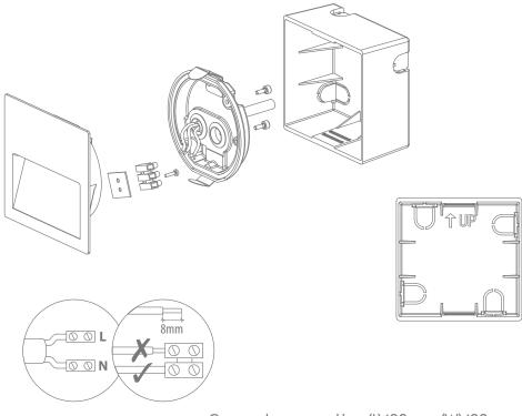
Cutout without recessed box: (L) 100mm x (W) 100mm Cutout with recessed box: (L) 110mm x (W) 110mm
