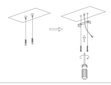
4. Properly align the mounting holes between back plate and mounting bracket, then lock them together with screw,
