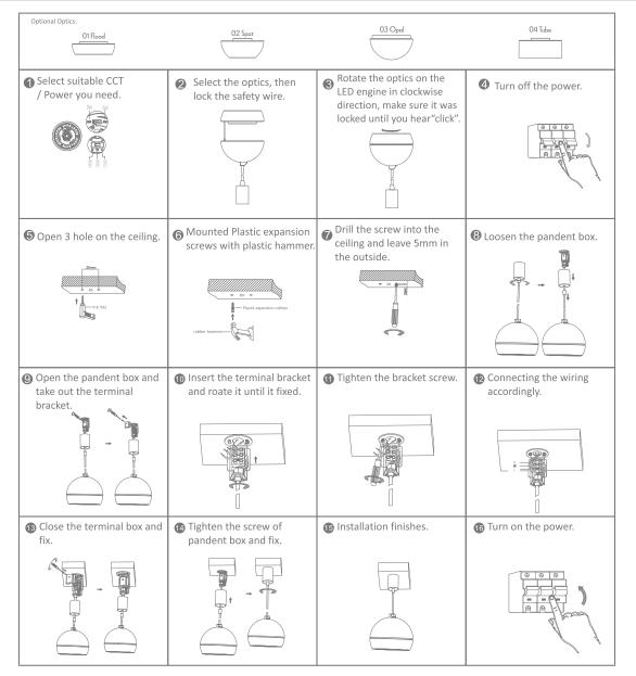
Note: -The lamp must be installed by professional electrician -Ensure the power supply is switched off before fitting this product
