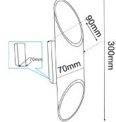
Depth: 30mm Mounting U Bracket: 60x20mm
