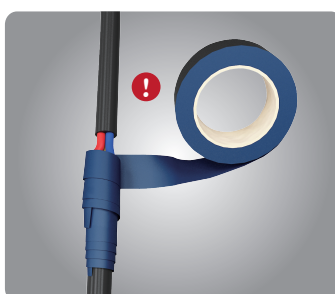
incorrect , using water-proof tape
