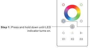
Step 2: Short press 5 times continuously to clear all bound lighting devices . LED indicator flashes 4 times for successful unbinding.
