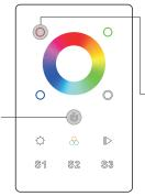
Step 2: From your zigbee controller or hub interface, choose to add device or accessory and enter Pairing mode as instructed by the controller.
