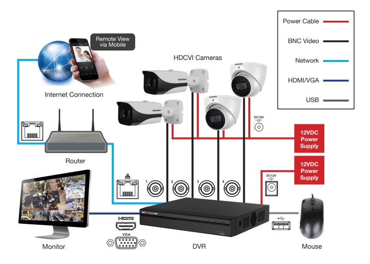
Fig. 1.2: System Setup Diagram
