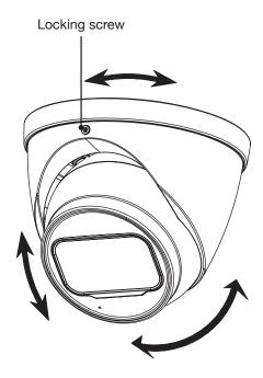
Fig. 3.4: Tri-axis fixed dome adjustment
