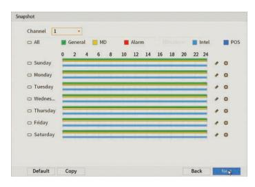
Fig. 2.14: Snapshot Schedule with Regular, Motion & Intelligent recording set to a 24/7 schedule.
