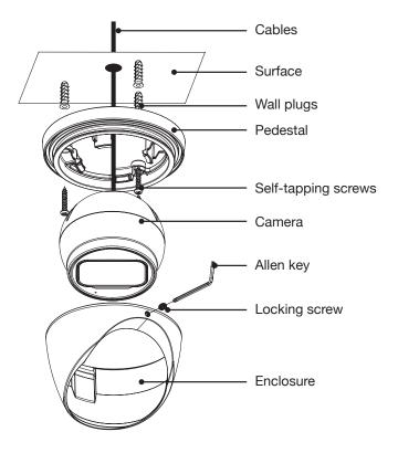
Fig. 3.3: Mounting diagram for fixed dome
