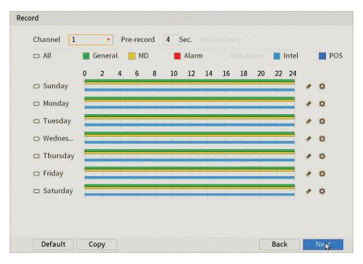
**Fig. 2.13:** Recording Schedule with Regular, Motion & Intelligent recording set to a 24/7 schedule.
