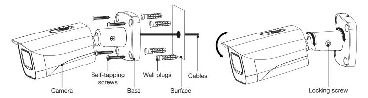
Fig. 3.1: Mounting diagram for fixed bullet
