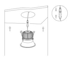
Connect the downlight with driver, hold back the spring clip then push the downlight into the hole.
