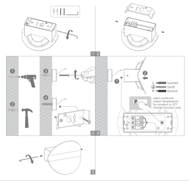
Note: -The lamp must be installed by professional electrician -Ensure the power supply is switched off before fitting this product
