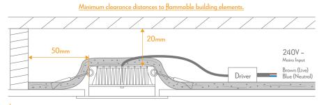
Note: The LED driver is NOT suitable for covering with insulation material. Warning-Risk of overheating or fire if the clearance distances are compromised. The flexible cable cannot be replaced, if this cable is damaged the luminaire will need to be replaced. The light source of this luminaire is not replaceable; at the end of life the whole luminaire should be replaced.
