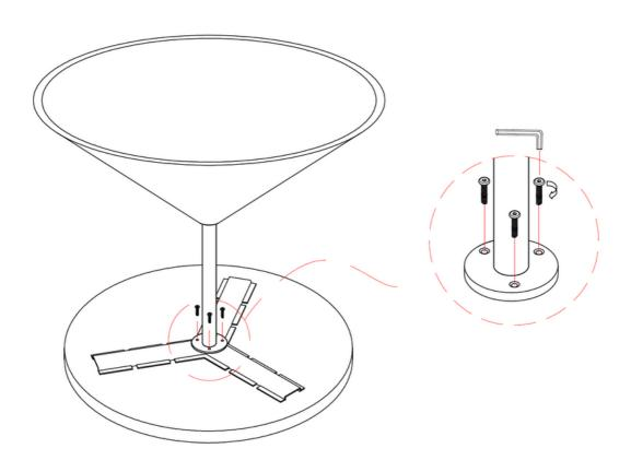
LINE UP THE TOP OF THE BASE PLATE (PART 1) TO THE HOLES IN THE TOP (PART 3)
